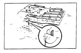
Disconnect the throttle cable from the cam and remove the valve body.
