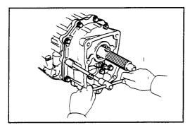
Install a new gasket and the transfer adaptor with the ten bolts.
