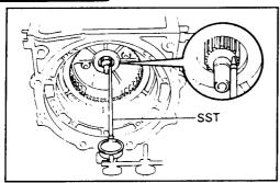
Using SST and a dial indicator, measure the thrust clearance of the input shaft. SST 09350-36010 (09350-06130)
