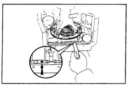
Hold first and reverse brake piston with hand, remove first and reverse brake piston by applying compressed air into the oil hole of the transmission case.
