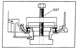
Using SST, compress the return spring. SST 09350-36010 (09350-06030)
