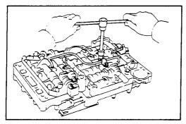
Install the tube clamp with the two wave washers and bolts.
