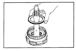
Remove the No.4 thrust washer.
