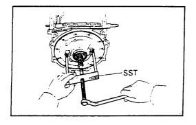
Using SST, remove the oil pump and gasket. SST 09350-36010 (09350-06140)
