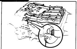
Connect the throttle cable to the cam.
