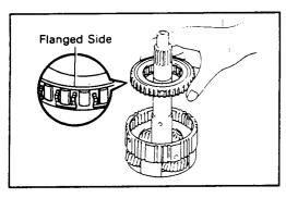
(c) Install the one-way clutch and outer race assembly, facing the flanged side of the one-way clutch upward.
