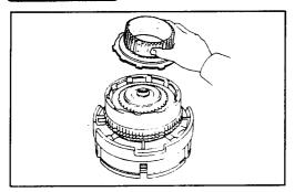
Remove the rear clutch hub.
