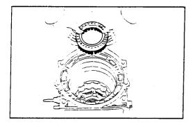
Place the return spring on the brake piston.
