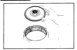
Remove the ring gear flange from the rear planetary ring gear.
