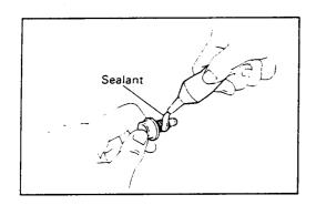
Apply sealant to the threads of the O/D case set bolts.
