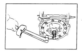
Place the gasket on the transmission case.
