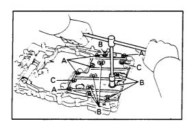
Install the body cover with the fifteen wave washers and bolts.
