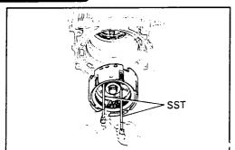
Install SST (two bolts) to the center support. SST 09350-36010 (09350-06140)
