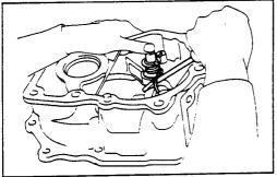
Hold the pawl shaft, hook another spring end to the pawl with a screwdriver.
