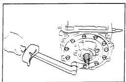
Remove the race from the oil pump cover. Select a race.
