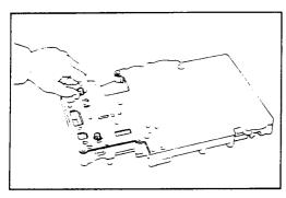
Temporarily secure the body plate with the two bolts.
