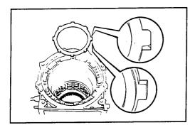
Install the flange, facing the rounded edge outward.
