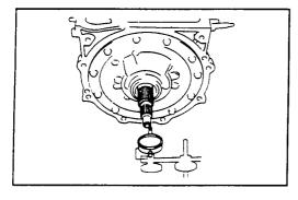
Using a dial indicator, measure the thrust clearance of the input shaft.
