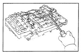
Using a large screwdriver, pry out the oil tube.
