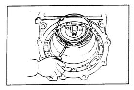
Using a screwdriver, remove the snap ring.
