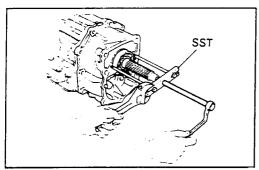
Using SST, remove the transfer adaptor together with the rear bearing.
