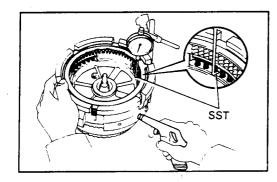
Using SST and a dial indicator, measure the piston stroke by applying and releasing the compressed air  $(4-8 \text{ kg/cm}^2, 57-114 \text{ psi or } 392-785 \text{ kPa})$  as shown.
