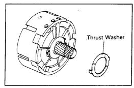
If the thrust clearance is greater than maximum, select and install a thrust washer.
