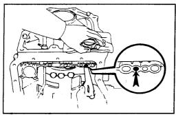
Remove the accumulator piston and spring by applying compressed air to the oil hole.
