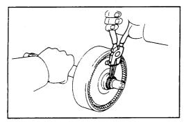
Install the ring gear and flange assembly.
