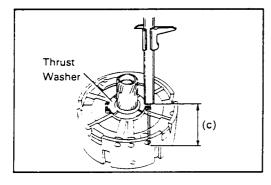
Turn over the center support together with the thrust washer, and place it on a flat surface.
