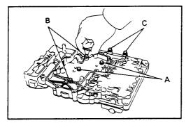
Temporarily install the six wave washers and bolts.
