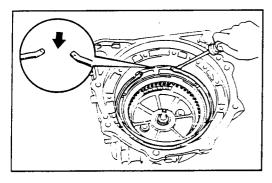
Using a screwdriver, install the snap ring.
