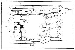
Temporarily install the lock-up relay valve body plate with the four short bolts.
