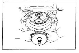
Remove the front clutch assembly.
