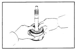
Remove the one-way clutch together with the outer race.
