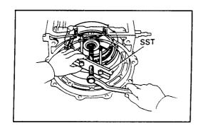
Using SST, remove the center support assembly from the transmission case.
