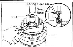
Place SST on the spring seat, and compress the return springs with a shop press.
