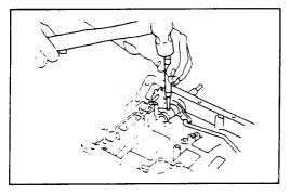
Using a pin punch, tap out the pin.
