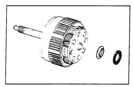
Remove the bearing and race from the O/D planetary gear or ring gear flange.
