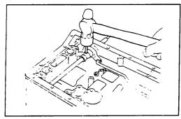
Using a hammer, tap in the pin with the slot at a right angle to the shaft.
