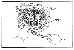
Using SST, remove the O/D case assembly. SST 09350-36010 (09350-06140)
