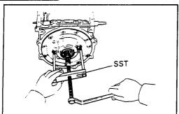
Using SST, remove the oil pump and gasket. SST 09350-36010 (09350-06140)  $\label{eq:sstar}$
