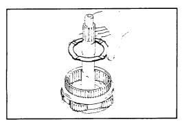
Remove the No.3 thrust washer.
