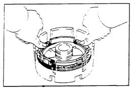
Push in the brake piston into the center support with both hands.
