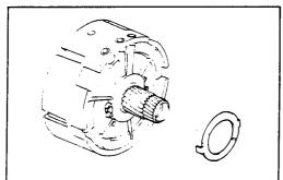
Remove the thrust washer from the center support.
