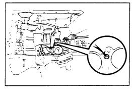
Remove the B<sub>0</sub> accumulator piston together with the B<sub>2</sub> accumulator piston by applying compressed air to the oil hole.
