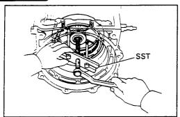
Using SST, remove the center support assembly. SST 09350-36010 (09350-06140)
