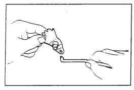
Connect the parking lock rod to the manual valve lever.
