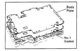
Place a new No.1 gasket and the body plate on the lower valve body.
