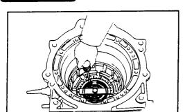
Using a screwdriver, install the snap ring.
