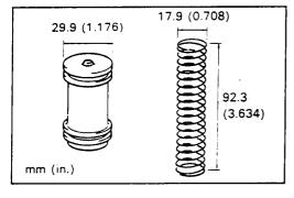
NOTE: Piston, spring diameters and spring free length are shown in the figure.
