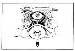
Remove the O/D planetary gear, direct clutch and one-way clutch assembly.
