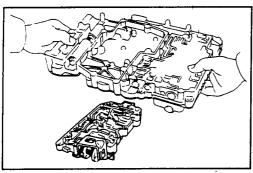
Place the lower valve body on the front upper valve body.
