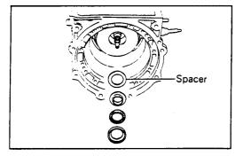
Remove the oil seal ring from the input shaft.
