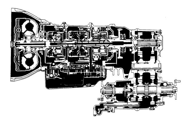
The A440F transmission is mainly composed of the torque converter, the overdrive (hereafter called O/D) planetary gear unit, 3-speed planetary gear unit, 2-speed transfer and the hydraulic control system.
