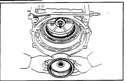
Install the ring gear assembly into the O/D case.
