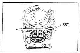
Coat new two O-rings with ATF, and install them to the brake piston.
