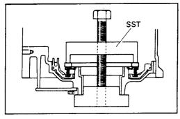
(c) Set SST on the spring retainer, and compress the return spring.
