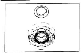
Remove the spring seat and twenty-four return springs.
