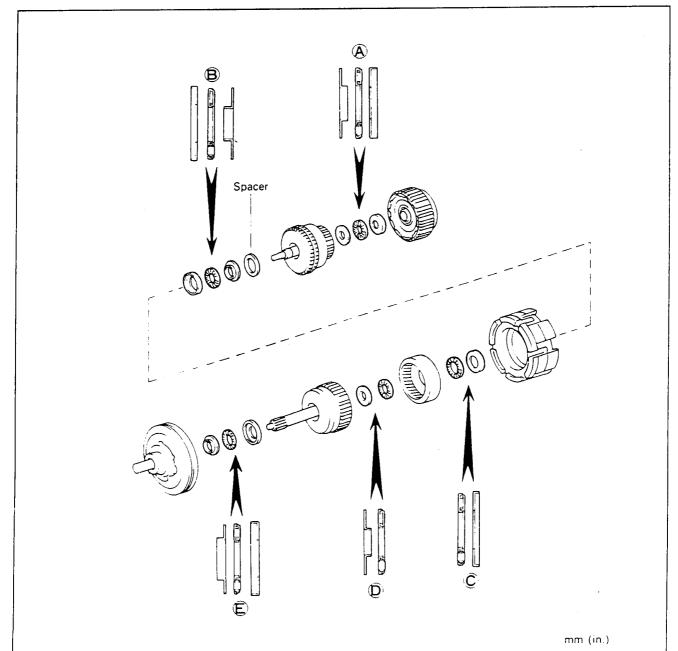
Bearing race diameter Thrust bearing diameter Front Rear Outside Inside Outside Inside Outside Inside 52.0 (2.047) 37.0 (1.457) A 34.7 (1.366) 52.0 (2.047) 32.8 (1.291) 50.4 (1.984) 50.4 (1.984) 32.8 (1.291) 37.0 (1.457) 52.0 (2.047) B 34.7 (1 366) 52 0 (2.047) Ĉ 52.0 (2.047) 37.0 (1.457) 34.7 (1 366) 52.0 (2.047) Ō 25.0 (0.894) 42.0 (1.654) 23.2 (0.913) 42.0 (1.654) 27 1 (1 067), 27 9 (1 098) or 28 3 (1 114) 48.0 (1.89) Ē 43.0 (1.693) 28.5 (1.122) 46 2 (1.819) 28 5 (1 122)
