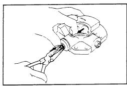
Using needle nose pliers, install the E-ring.
