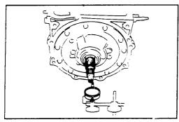
Using dial indicator, measure the thrust clearance of the input shaft.
