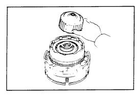
Remove the front clutch hub.
