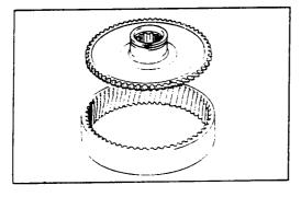
Remove the ring gear flange.
