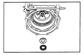
Remove the thrust bearing and race from the O/D case or ring gear flange.
