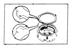
(b) Install the flange, facing the rounded edge upward. NOTE: If the flange is step-edged, install the flange with the step-edge, facing downward.
