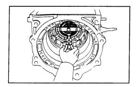
Using snap ring pliers, remove the snap ring.
