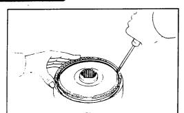
Using a small screwdriver, install the snap ring.
