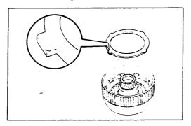
Install the flange, facing the rounded edge upward.
