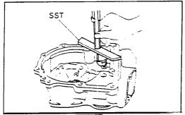
Using SST and calipers, set the pawl bracket so that so the distance between the transfer adaptor surface and the top of the bracket tab is specified distance.
