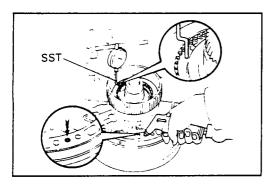
Using SST and a dial indicator, measure the piston stroke by applying and releasing the compressed air (4 – 8 kg/cm², 57 – 114 psi or 392 – 785 kPa) as shown.
