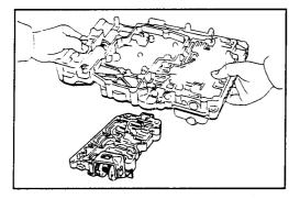
Remove the front upper valve body by lifting up the lower valve body.
