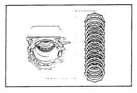
(b) Remove the flange, six discs, six plates and cushion plate.
