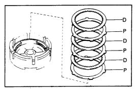
Remove the flange, three discs and three plates.
