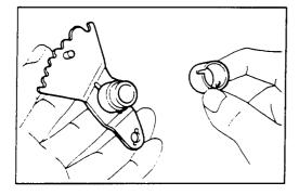
Assemble a new spacer to the manual valve lever.
