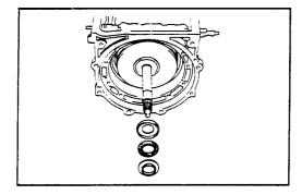
Remove the two races and thrust bearing from the O/D direct clutch drum or oil pump.
