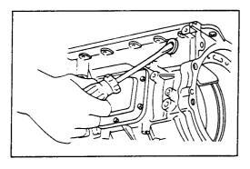
Using a screwdriver, pry out the two oil seals.
