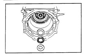
Remove the two races and thrust bearing from the rear clutch drum or front clutch hub.
