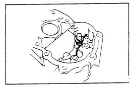
Insert the spring end to the hole of the transfer adaptor, and install the pawl shaft.
