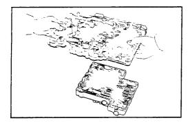
Remove the rear upper valve body by lifting up the lower valve body.
