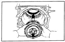
Remove the planetary gears, one-way clutch and output shaft assembly.
