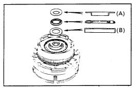
Remove the two races and thrust bearing.
