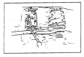
Using a large screwdriver, remove the oil tube by prying both tube ends.
