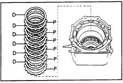
Install the six plates and six discs in order:
