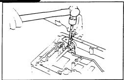
Match the spacer hole to the lever calking hollow and calk the spacer to the lever.
