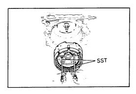
Remove the two races, thrust bearing and spacer from the front clutch drum or O/D case. Select a spacer.
