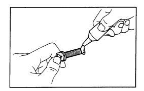
Apply sealant to the bolt threads.
